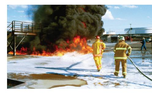
Niagara<sup>C6</sup> 3-3 is a superior quality Alcohol Resistant Film-Forming FluroProtein (AR-FFFP) fire fighting foam concentrate at 3% induction rate for extinguishing and securing both flammable hydrocarbon and polar solvent liquid fires.
