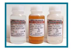
Before taking a sample, activate the foam system long enough to remove standing columns of water (which otherwise would contribute to a diluted produced foam sample), and sample when the system is in equilibrium.
